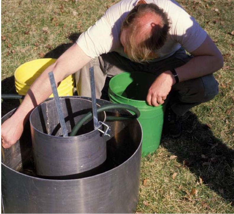
Traditional ASCE double-ring infiltrometer.
