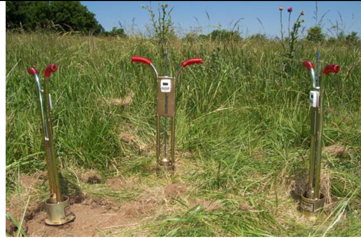
Set of three Turf-Tec infiltrometers for infiltration measurements in pre-development soils.
