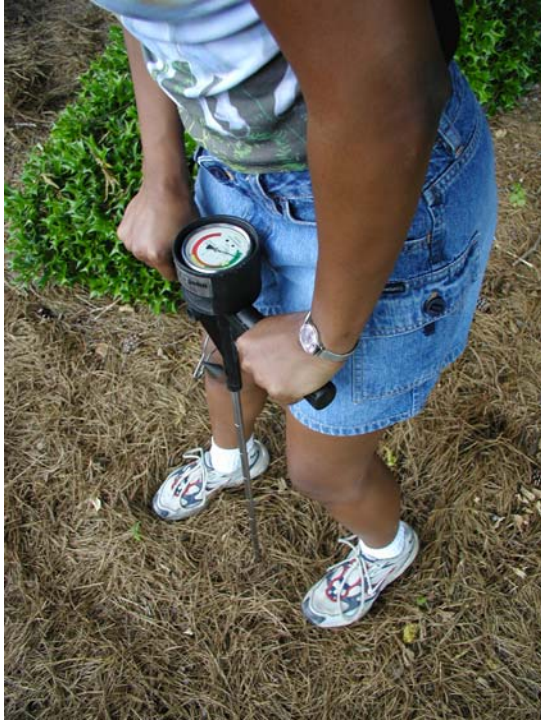
Cone penetrometer measurement.
