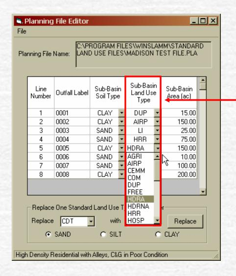
Use the Pull-Down Menu to Select Subbasin Land Use Type. The land uses are referenced from the folder that was originally selected in the Main Window of the Batch Editor.
