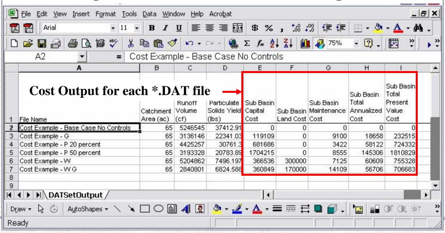
The shows the output for each Control Device when the Cost File is run through the Batch Editor. Import the output file 'DATSetOutputCostDetail.CSV' into Microsoft Excel.
