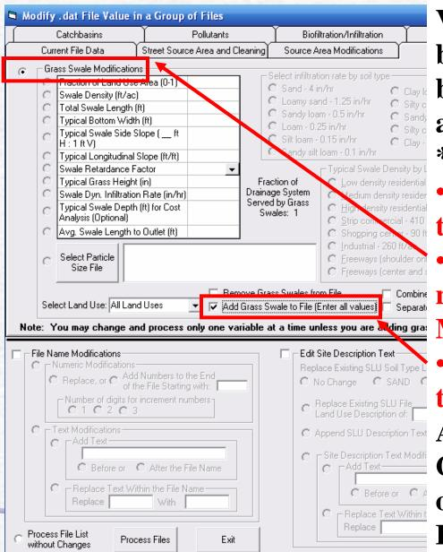
Various Control Devices can be added to \*.DAT files in a batch. This example will show adding Grass Swales to a \*.DAT file.
