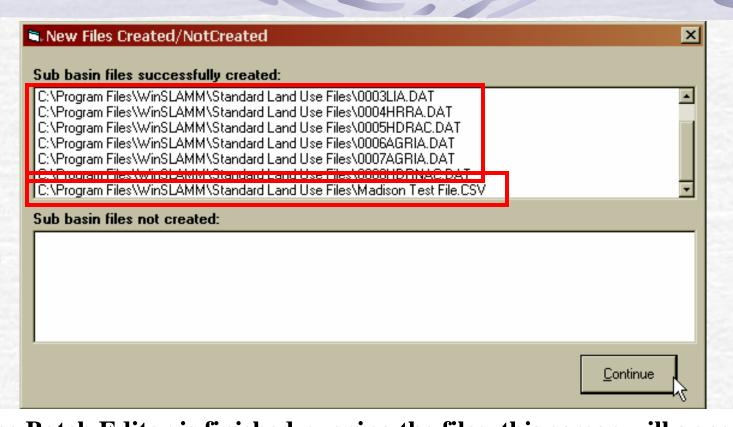
When the Batch Editor is finished running the files, this screen will appear. The top window shows each \*.DAT file that was created and the commaseparated-value file (.csv) with the outfall summaries for each subcatchment. This \*.csv file can be imported into Microsoft Excel for analysis. The bottom window will show the \*.DAT files that could not be created. The user will need to check the files in the bottom window and modify them so they can be run by the Batch Editor.
