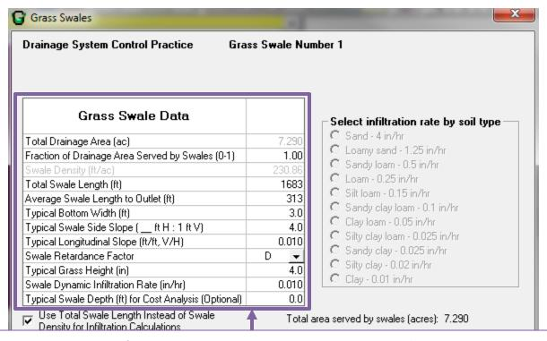
Enter the data for each grass swale. The "Average Swale Length to Outlet" will automatically populate after other swale data is entered.
