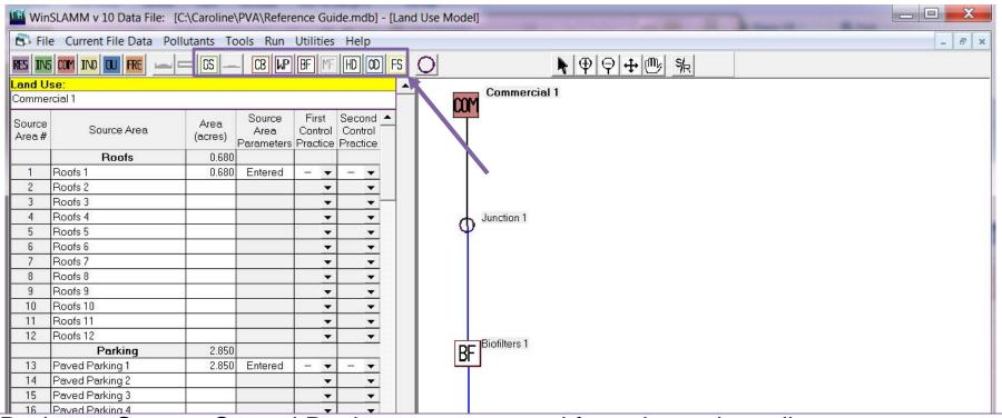
Drainage System Control Devices are accessed from the main toolbar.
