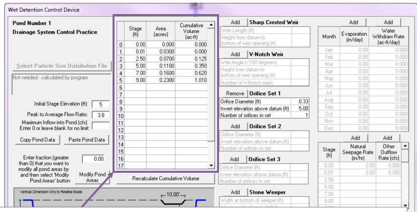
Enter the Stage Area Data for the pond. At least five stage increments must be entered. The area of the pond at the datum must be zero. Enter the first stage of the bottom of the pond as 0.01.
