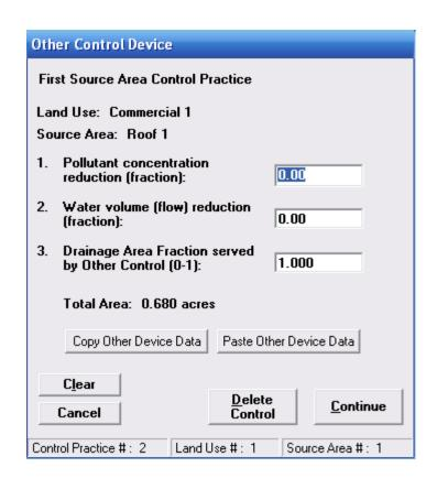
Enter the Percent Reduction in Pollutant Concentration and Runoff, and the Fraction of the Area served by the Control Device. The percent reduction will be applied uniformly to the Pollutant Load and Runoff Volume generated.
