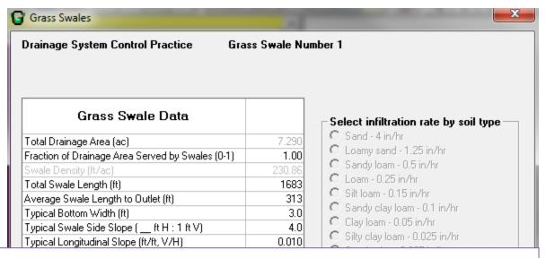
If the swale density and swale length are unknown, select a value based on land use.
