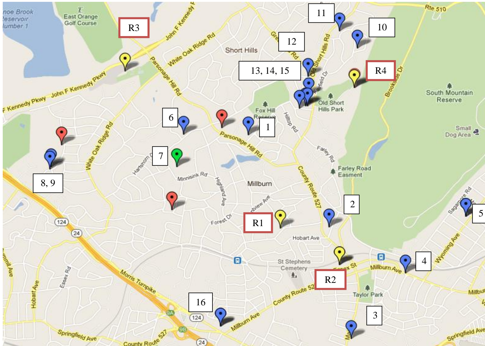
Figure 4.4. Location of dry wells (blue icons), rain gauges (yellow icons), and water quality samplers (red icons for dry wells and green icon for cistern)(source: maps.google.com).
