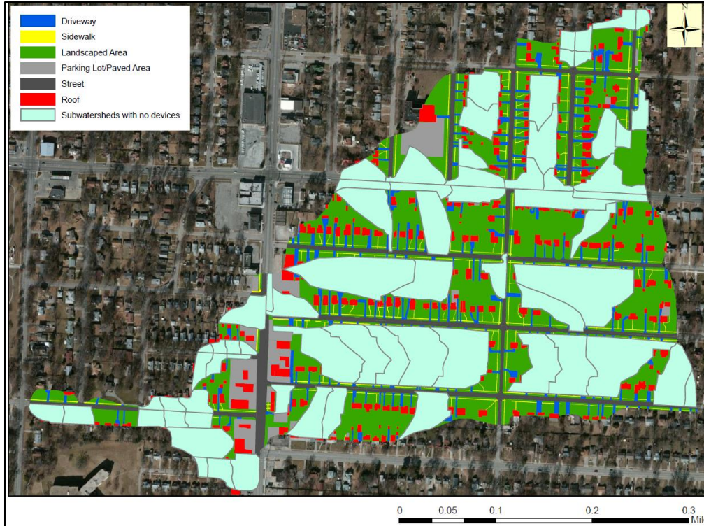
Figure 3.20. Map of test (pilot) area showing surface characteristics of areas receiving stormwater treatment.
